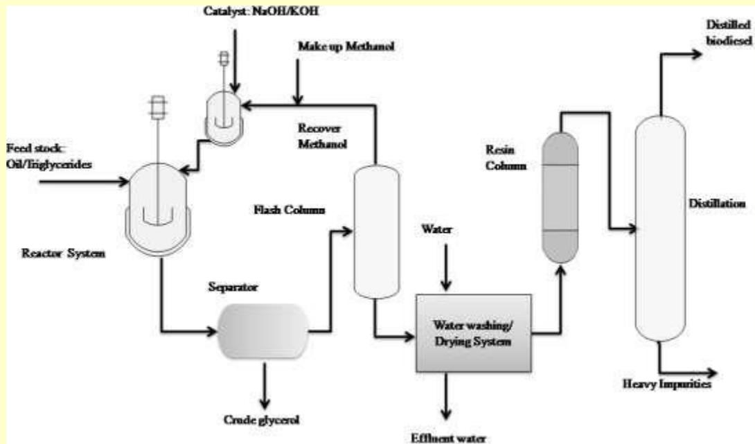
**Figure 2: Simplified process flow diagram for conventional homogeneous catalytic biodiesel process**
